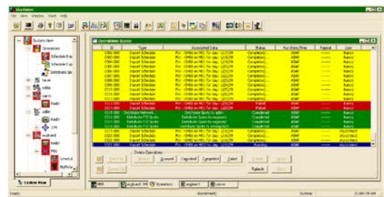
Operations Queue View: Displays all operations for a configured set period of time—primarily used to monitor or edit schedule operations.
